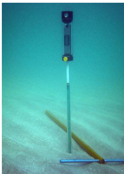
Figure 4.4. Example of SediMeter installation (Lindorm 2009a)
