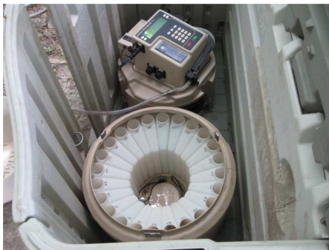
Figure 4.3. Sigma sampler: the computer and pump are displayed in the top of the picture while the bottles used to store the samples are on the bottom
