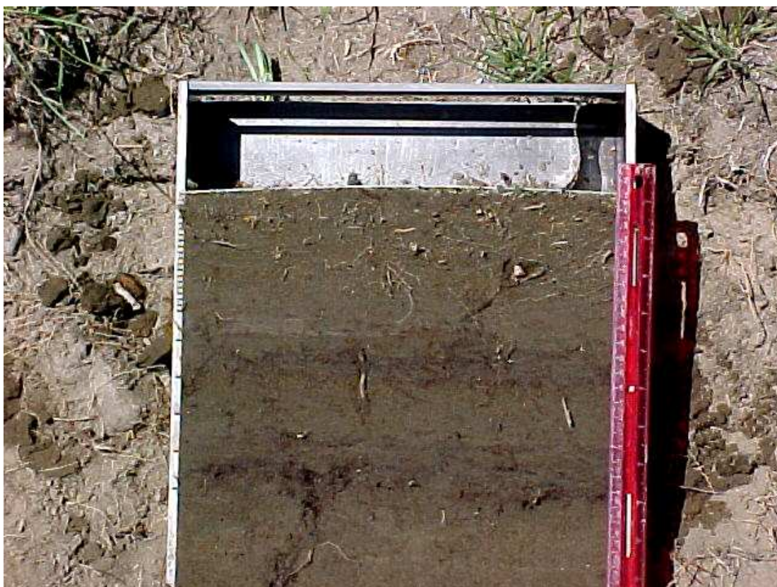
Figure 4.9. Upland source sample prepared for division into 5-cm increments
